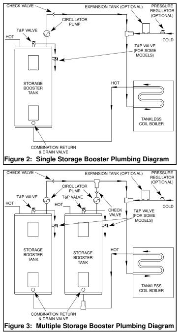
tem, check valves must be installed to prevent the circulator from pumping hot water into another tank and overheating it.
